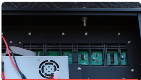
Move the power supply for access
