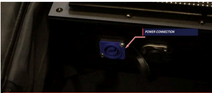
Locate the blue power connection
