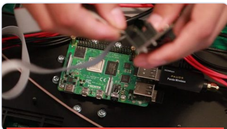
Lift straight off the header pins
