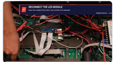
Reconnect until the clip engages
