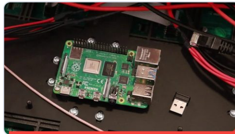
Match the 40-pin-header orientation
