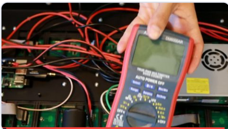
Set the multimeter to DC volts
