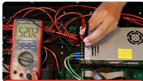
Probe the DC output terminals
